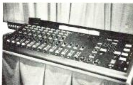
This Langevin console has nine channels in and four out. Circle 78 on Reader Service Card.
