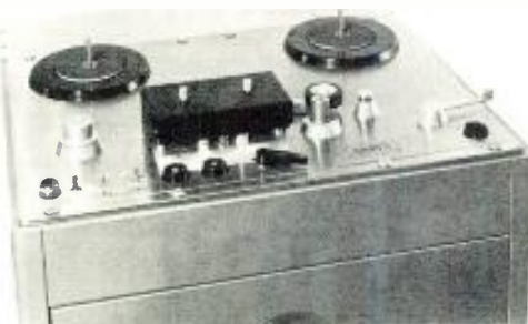
The Ampex BML-200's bin slopes and has a transparent front. Electronics are below, including a pump and the power supply. The slave unit deck can have guides and heads interchanged.
