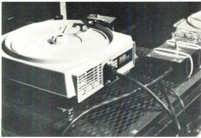
Figure 7. One of the standard projectors. Note the microswitch mounted at the zero position on the unit. At the right is the control box.
