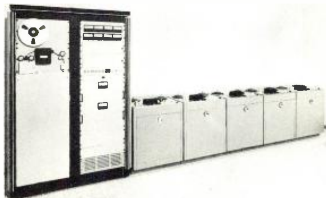
A Vega master, electronics rack, and five slaves. The tape-loop rack is below the transport, while the master electronics are in the adjoining rack.
