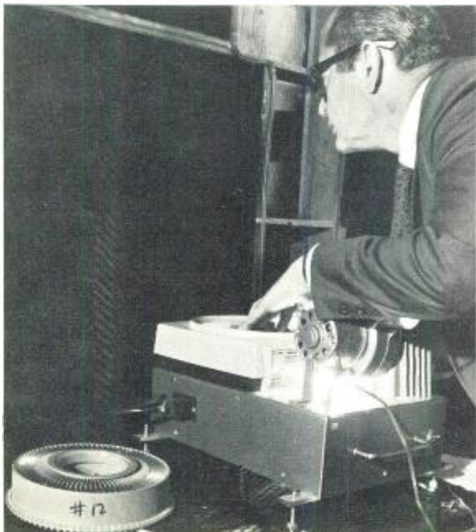
Figure 9. Technical director Stan Goldstein is shown adjusting the alignment of a projector with an SMPTE slide.
