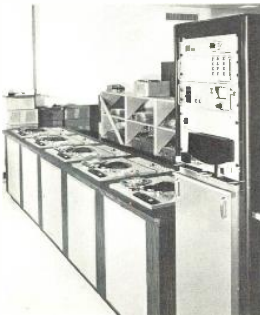
An actual installation of the GRT-260 system with five slaves. The solid-front tape bin is below the transport of the master, with some control electronics above. (continued on page 38)
